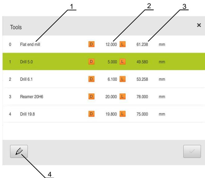
Figure 29: Tool table with tool parameters
