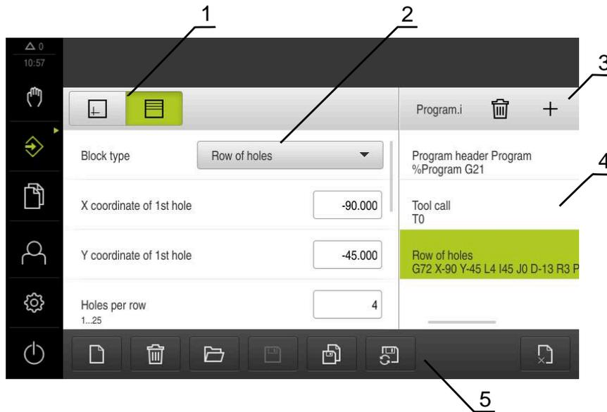
Figure 59: Example of a program in the **Programming** operating mode
