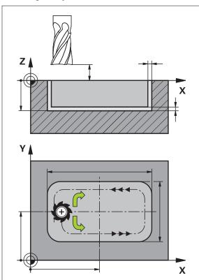
Figure 58: Schematic display of the rectangular pocket block
