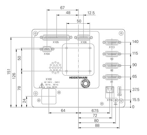
Figure 37: Housing dimensions of the rear panel for devices with ID 1089179-xx  $\,$
