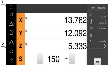
Figure 3: User interface (in Manual operation mode)
