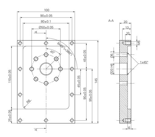
Figure 62: Example workpiece- technical drawing
