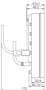
Figure 35: Housing dimensions for devices with ID 1089179-xx
