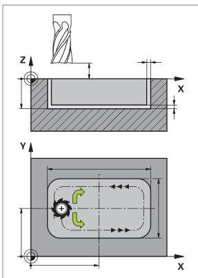
Figure 47: Schematic display of the rectangular pocket block
