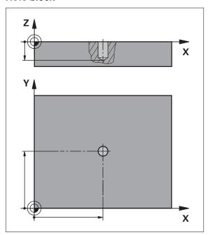
Figure 44: Schematic depiction of the **Hole** block
