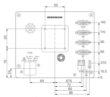
Figure 36: Dimensions of the rear panel for devices with ID 1089178-xx
