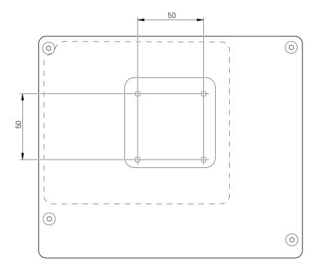
Figure 15: Dimensions of rear panel of the product
