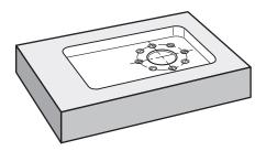
Figure 68: Example workpiece – drilling a circular hole pattern
