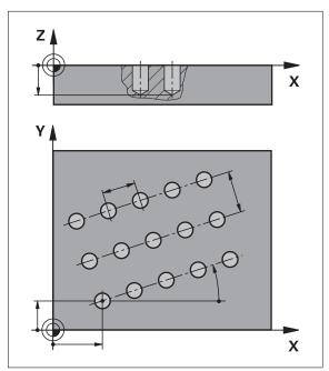
Figure 46: Schematic display of the row of holes block
