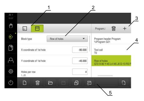
Figure 59: Example of a program in the **Programming** operating mode
