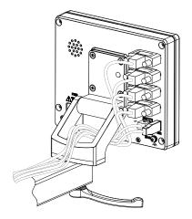
Figure 23: Cable routing on Multi-Pos holder
