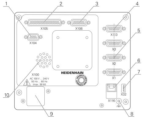
Figure 25: Rear panel on devices with ID 1089179-xx
