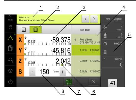
Figure 48: Example of a block in MDI mode
