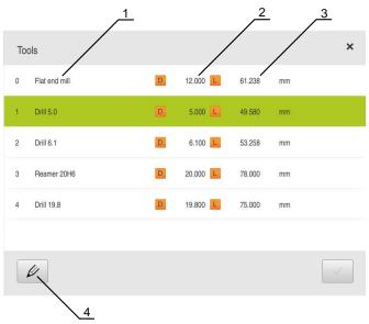
Figure 29: Tool table with tool parameters
