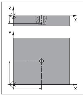
Figure 55: Schematic depiction of the **Hole** block
