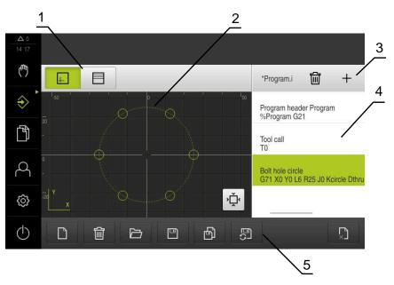
Figure 9: Programming menu with opened simulation window
