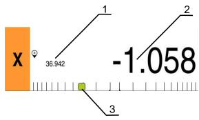
Figure 50: **Distance to go with position** view with graphical positioning aid
