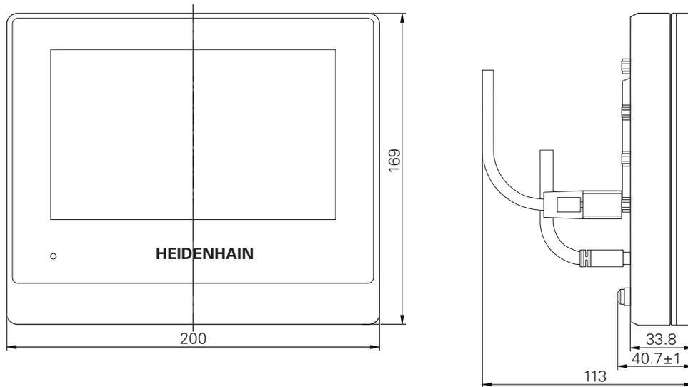
Figure 45: Housing dimensions for devices with ID 1089178-xx
