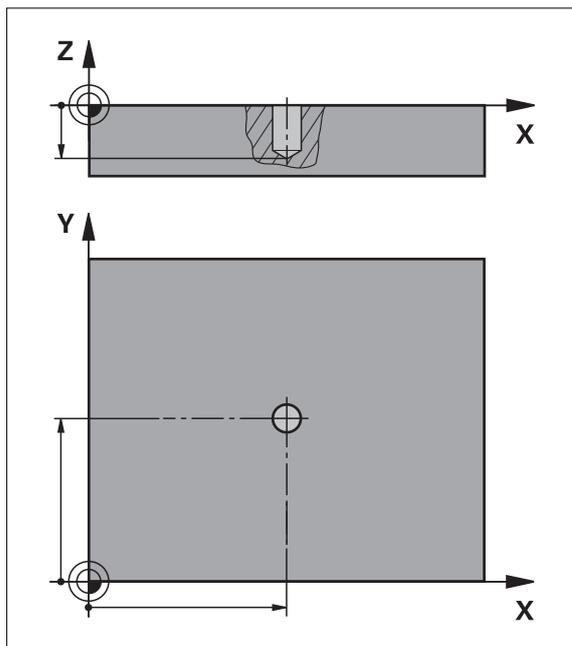
Figure 64: Schematic depiction of the **Hole** block
