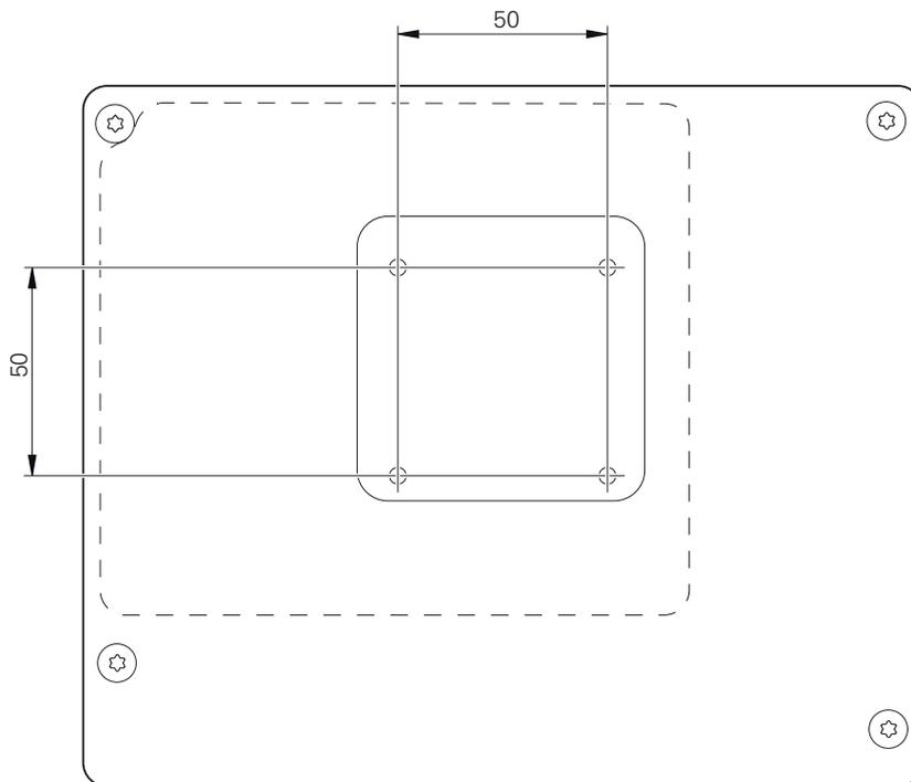
Figure 12: Dimensions of rear panel of the product
