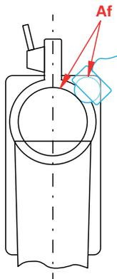
Figure 30: Relationship of the angular encoder relative to the column axis
