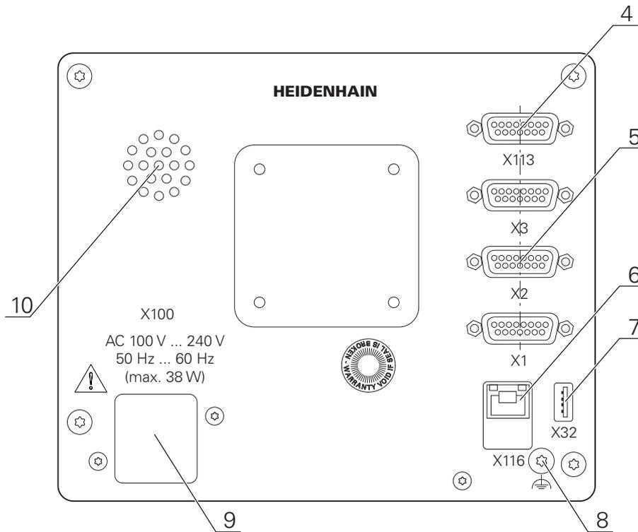
Figure 21: Rear panel on devices with ID 1089178-xx
