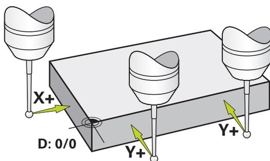
Figure 71: Example workpiece – finding the preset
