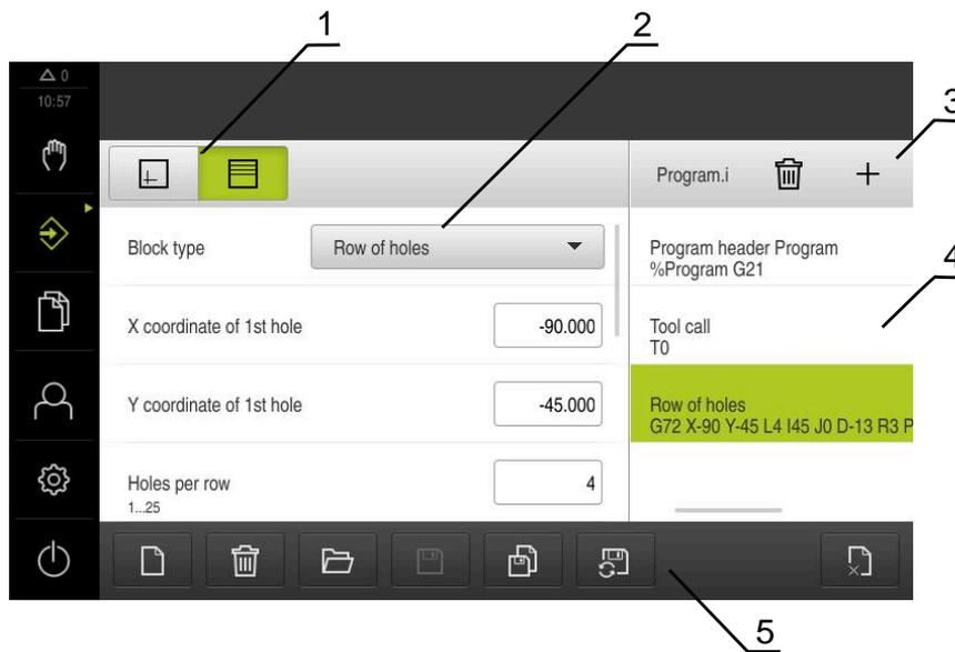
Figure 67: Example of a program in the **Programming** operating mode
