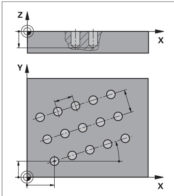
Figure 57: Schematic display of the row of holes block
