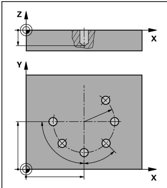
Figure 65: Schematic display of the bolt hole circle block
