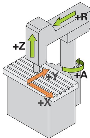
Figure 25: Design of a rapid radial drilling machine
