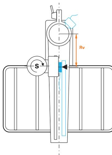
Figure 29: Plan view of a radial drilling machine
