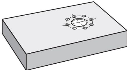
Figure 74: Example workpiece – drilling a bolt hole circle
