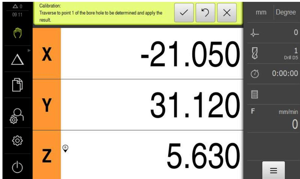
Figure 37: Step for moving to calibration positions
